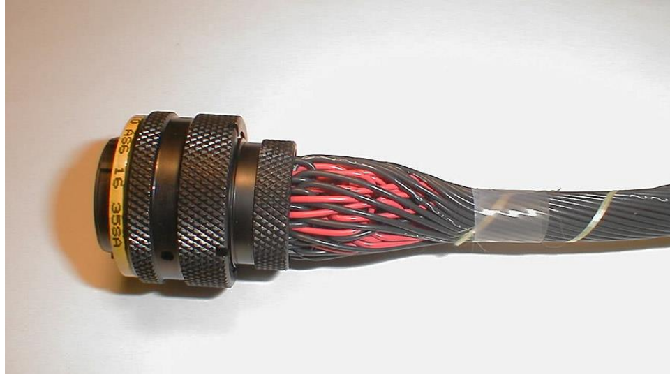
Figure 29: Example of concentric twisting and service loops (reprinted with permission from RB Racing)
