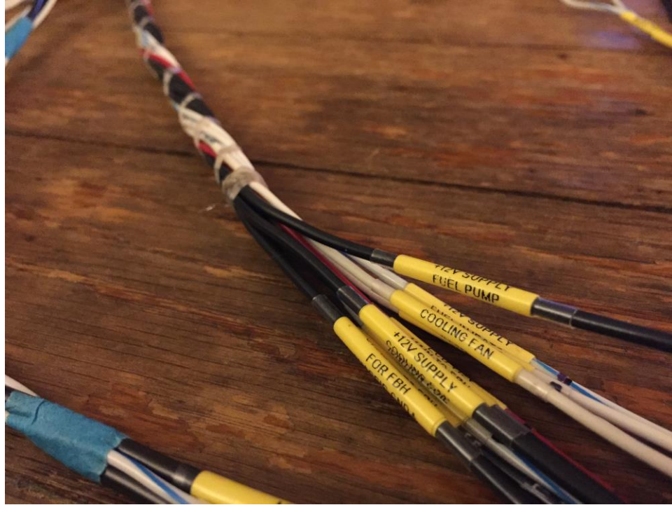
Figure 26: Example of labels with clear heat-shrink on each wire
