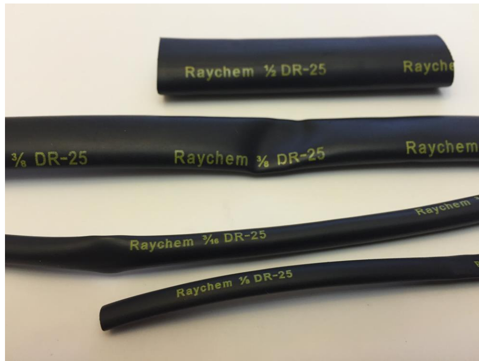
Figure 14: Example of the Raychem DR-25 heat-shrink tubing
