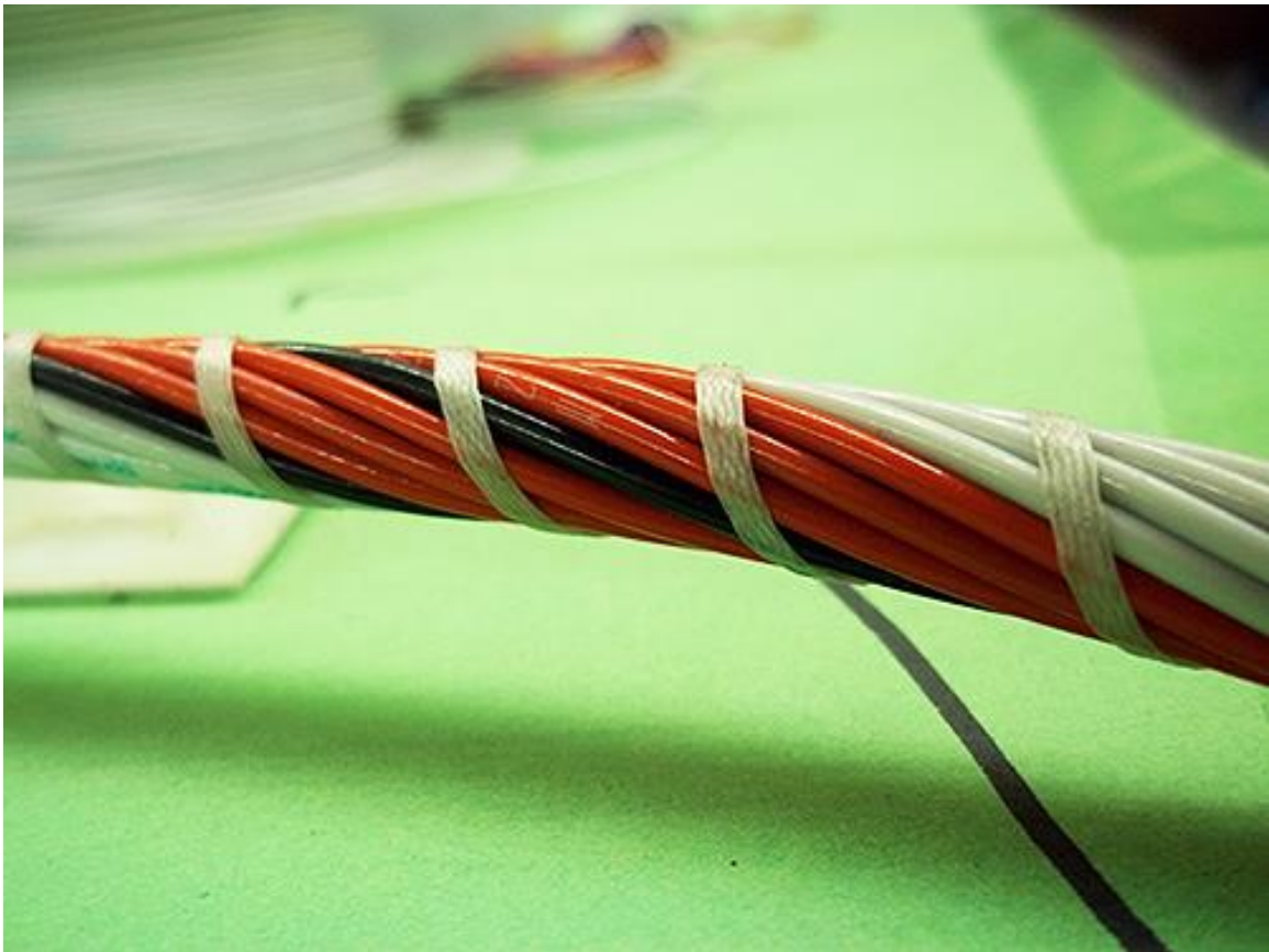
Figure 32: Example of concentrically twisted and laced section of wiring harness (reprinted with permission from RB Racing)
